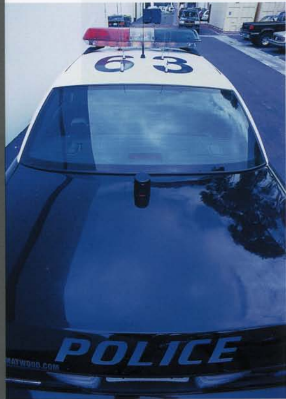
The vehicular repeater's antenna is mounted on the trunk lip to prevent interference from the mobile transmitting antenna mounted on the vehicle's roof.
